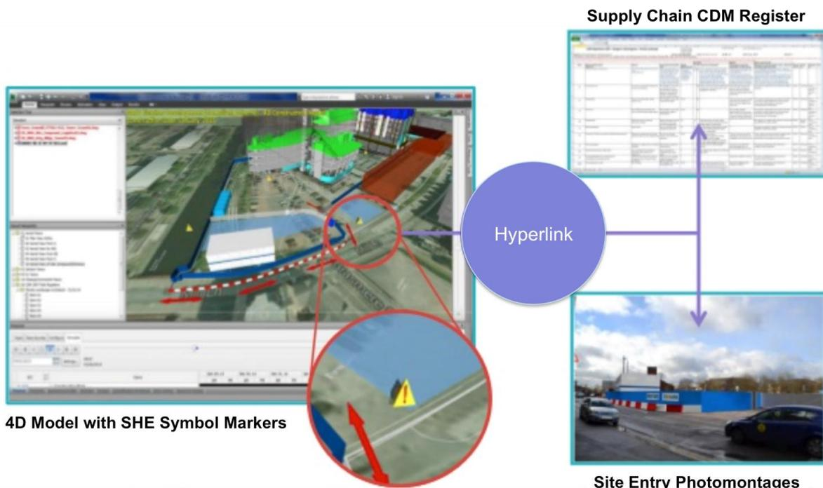
Figure A-9 Planning to mitigate health and safety risks using BIM – Balfour Beatty (2015)
